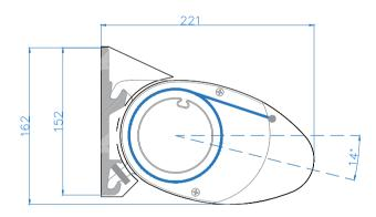
A pitch of 14° (25cm slope per metre) or greater is required to ensure rain water run off
