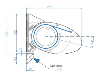
A pitch of 14° (25cm slope per metre) or greater is required to ensure rain water run off
