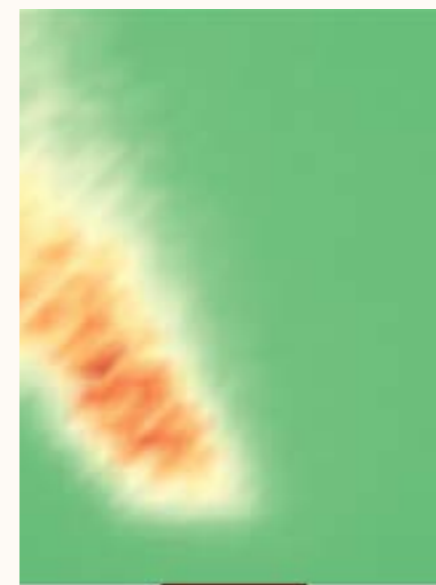
'perforate' infill (contrasol perforated - approx 15%) daylight lux plot, sunny sky
